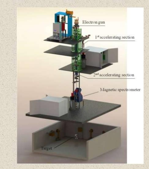
The main part of the IREN facility is a linear electron accelerator. The bunched electron beam generates bremstruhlung in the tungsten target and it produces the neutron pulses via  $(\gamma,n)$ -reaction in the same target.
