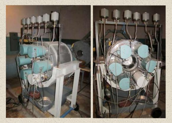
Detector contains 6 sections forming together the cylinder with the channel along the beam neutron direction. Diameter of the channel is 300 mm, external diameter of the detector is 730 mm, length 600 mm. Total volume of liquid scintillator is 250 liters. There are photomultipliers in both ends of each section. The signals from two photomultipliers of each section are summarized on output load resistor.
